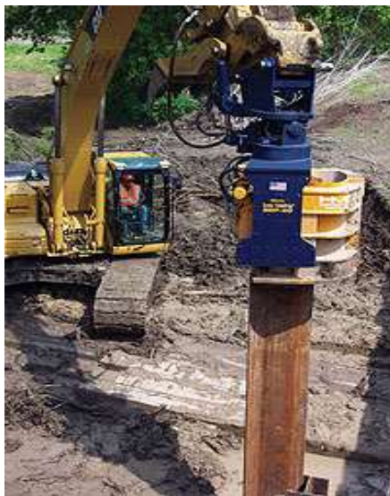
Pile Driver (Vibratory) (Caterpillar 235)
